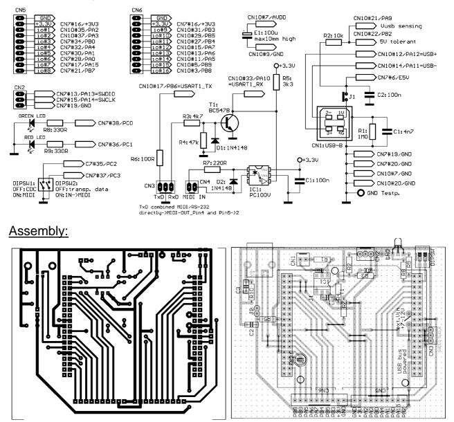
In contrast to the previous hardware version, V<sub>USB</sub> is connected permanently with PA9. So it is possible (but less recommended), to supply the board with external power 7..12V DC. Due to Veroboard limited wiring resolution, the wire is put via PB2, which is HiZ input and 5V tolerant. J1 is only used for measurement of supply current. For longterm practical use it should be shorted with solder.
