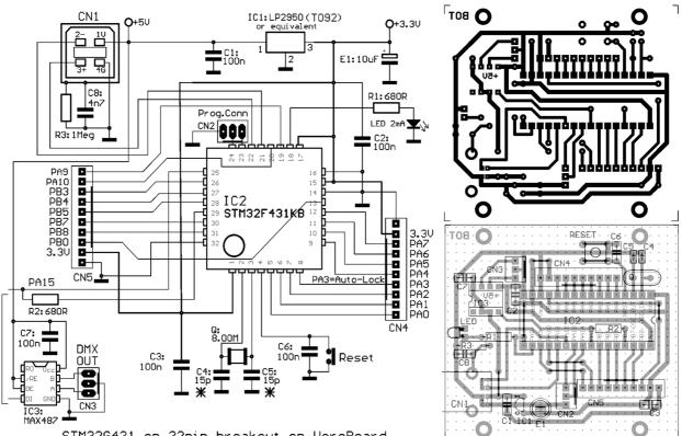
STM32G431 on 32pin breakout on VeroBoard
